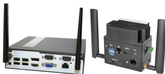
DL10J (see left) and EN01J4 (see right) with installed cellular antennas.
