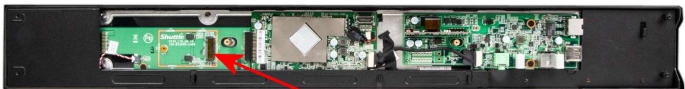
Top view – the location of the M.2 slot for the LTE adapter card
